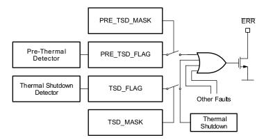
Figure 18. Thermal Fault Report Topology
