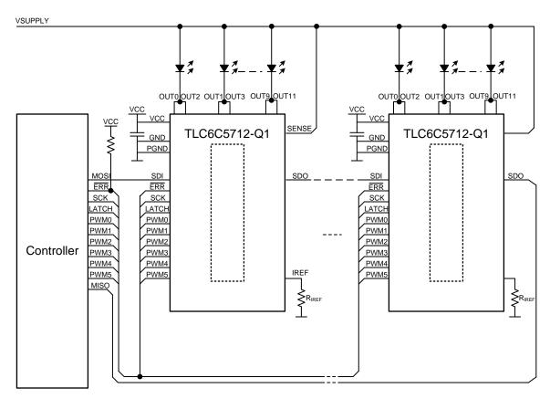
Figure 109. Application Schematic for TLC6C5712-Q1 Devices With Parallel Outputs
