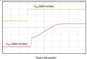
$R_L = 6.2 \Omega$ , 1- $\mu$ F output capacitor
