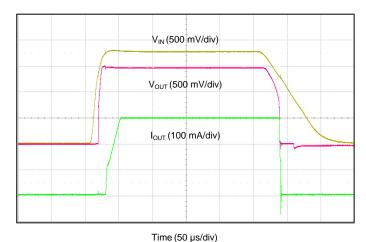
Figure 23. 1.8-V to 1.5-V Regulation at 300 mA
