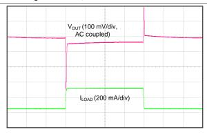
$V_{IN} = 3.8 \text{ V, no output capacitor,} \\ \text{output current slew rate} = 0.25 \text{ A/}\mu\text{s}$
