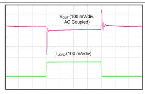
$V_{IN}=3.8\ V,1\text{-}\mu\text{F}\ \text{output}\ \text{capacitor,}$  output current slew rate = 0.25 A/ $\mu\text{s}$
