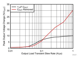
Output current stepped from 50 mA to 300 mA, output voltage change measured at positive dI/dt
