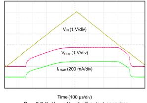
$R_L = 6.2 \Omega$ ,  $V_{EN} = V_{IN}$ , 1- $\mu$ F output capacitor Figure 17.  $V_{IN}$  Power-Up and Power-Down
