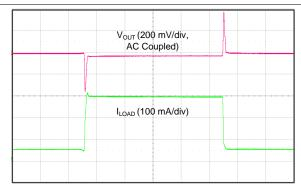
$V_{IN} = 2.0 \text{ V}, \text{ no output capacitor}, \\ \text{output current slew rate} = 0.25 \text{ A/}\mu\text{s}$
