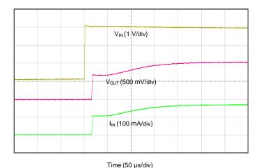
Figure 25. No Inrush Startup, 3.0-V to 1.0-V Regulation
