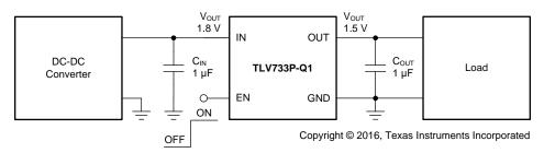
Figure 22. DC-DC Converter Post Regulation
