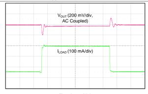
$V_{IN} = 2.0 \text{ V, } 1\text{-}\mu\text{F output capacitor,} \\ \text{output current slew rate} = 0.25 \text{ A/}\mu\text{s}$
