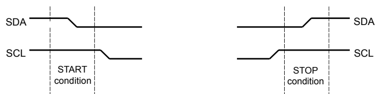
Figure 16-3. START and STOP Conditions
