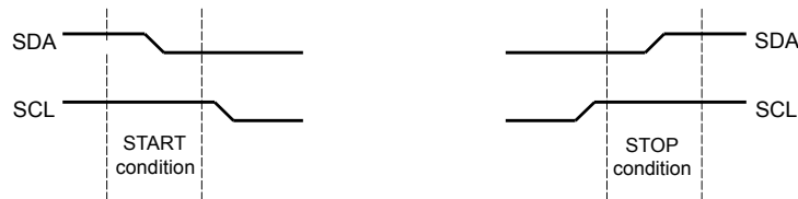
Figure 18-3. START and STOP Conditions
