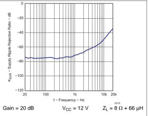
Figure 14. Supply Ripple Rejection Ratio vs Frequency
