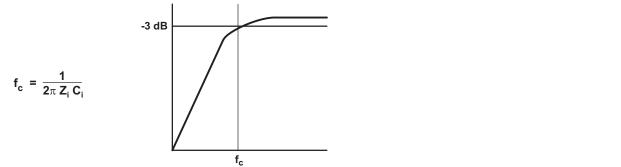
The value of  $C_I$  is important, as it directly affects the bass (low-frequency) performance of the circuit. Consider the example where  $Z_I$  is 60 k $\Omega$  and the specification calls for a flat bass response down to 20 Hz. Equation 3 is reconfigured as Equation 4.
