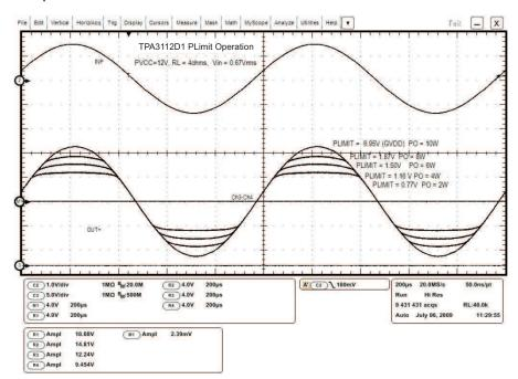
Figure 15. Plimit Circuit Operation
