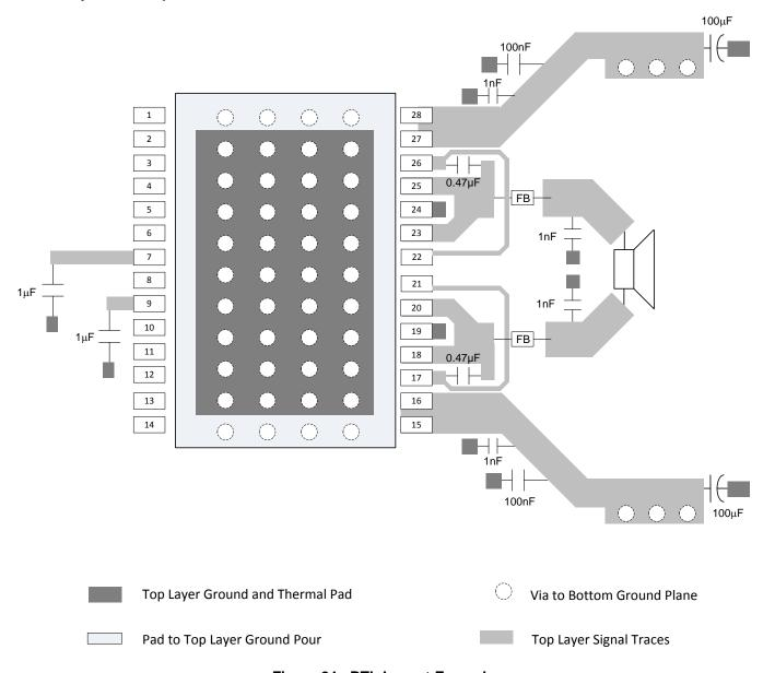
Figure 24. BTL Layout Example
