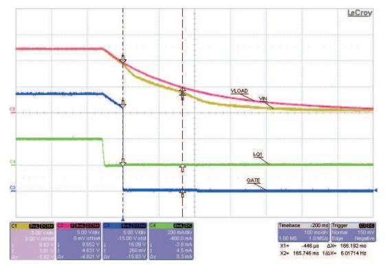
Figure 12. B2B Performance with 200-mA Load
