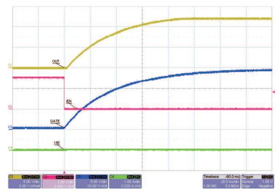
Figure 8. Start-Up With Slew Rate Control (C<sub>EXT</sub> = 0.1  $\mu$ F)
