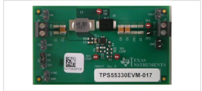
Integrated 5-A, 24-V Wide Input Range Boost DC/DC Regulator Evaluation Module
