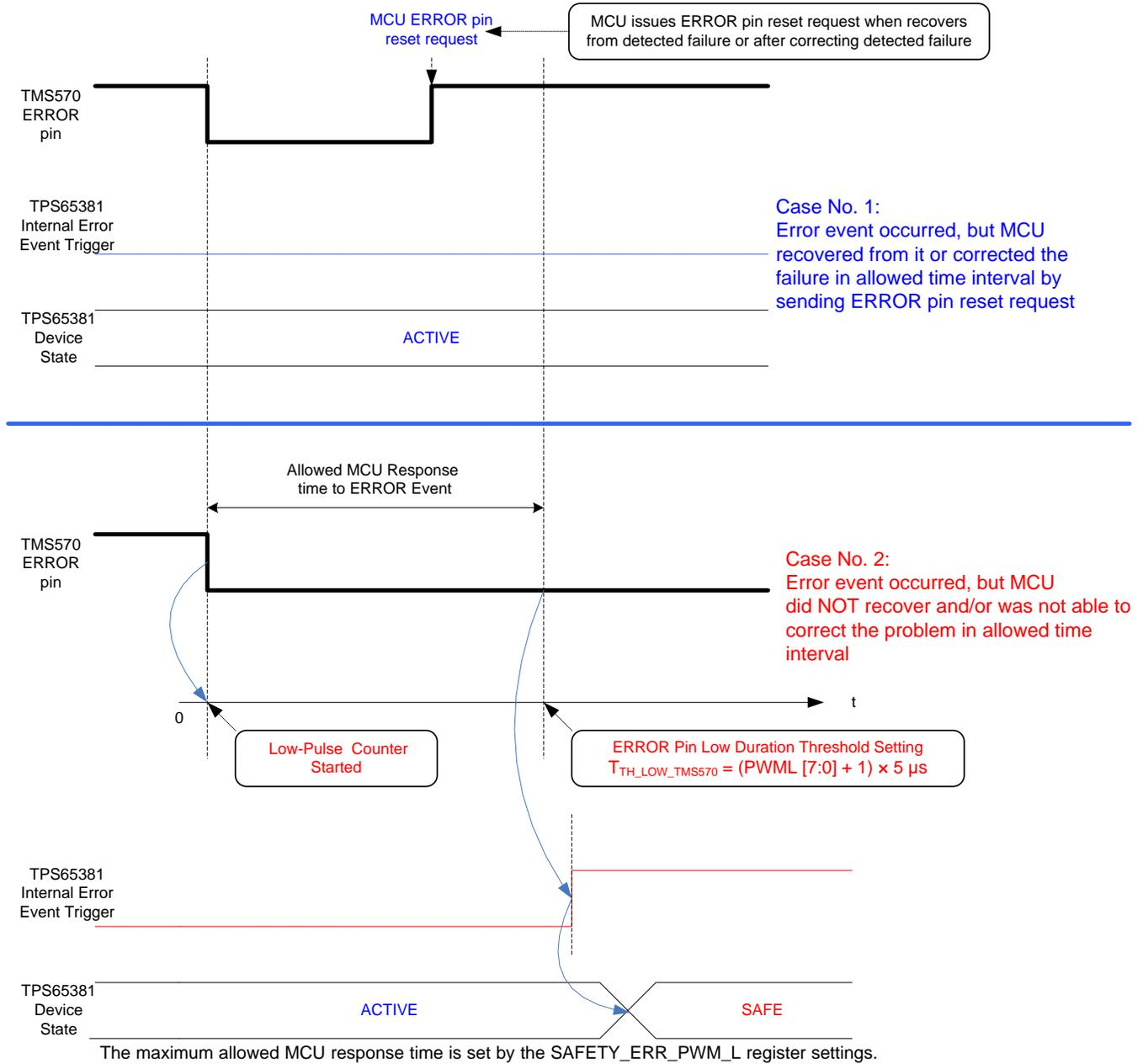
**Figure 5-11. Error-Detection Case Scenarios for the TMS570 MCU**
