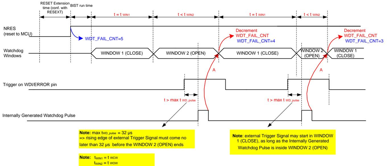
Note: When a *good event* is received in WINDOW 2 (OPEN), 1 system clock-cycle (250 ns, typical) later the next watchdog sequence begins. Therefore the actual length of WINDOW 2 (OPEN) depends on when the MCU sends the *good event*.
