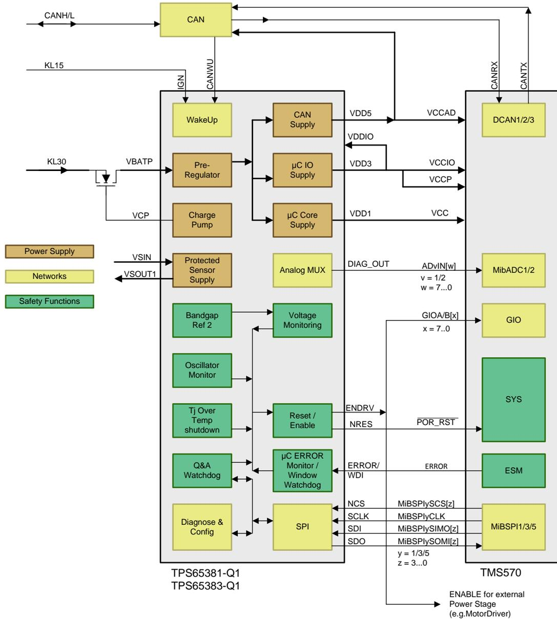
Figure 6-9. Example TPS65381-Q1 With TI's TMS570LS
