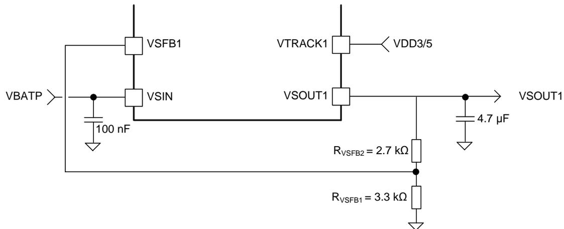
Figure 6-5. VSOUT1 Design—Tracking, With Gain (VDD3/5)
