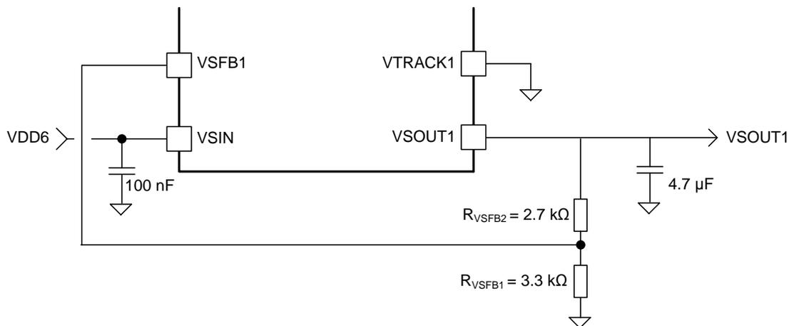
Figure 6-7. VSOUT1 Design—Non-Tracking
