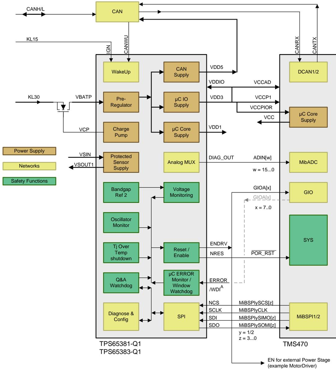
The ERROR/WDI pin can be configured as an input for the  $\mu$ C ERROR monitor (TMS570 dual core) or as a window watchdog input (TMS470 single core).
