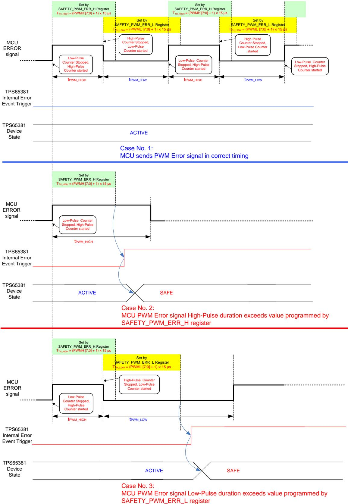
Figure 5-12. ERROR Pin Monitor – PWM Mode
