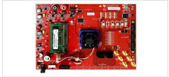
Top View of TSW1400EVM High Speed Data Capture and Pattern Generation Platform
