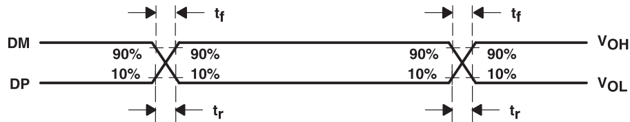
Figure 2. Differential Driver Timing Waveforms
