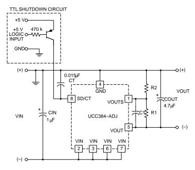
Figure 8. TTL Controlled Shutdown Circuit for the UCC384
