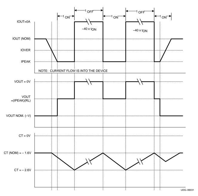
**Figure 5. Short Circuit Timing**
