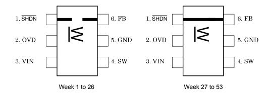
Note: This IC could be destroyed in some case if amounted in 180° inverse direction. Please be careful about IC direction in mounting.
