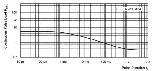
Maximum pulse load, continuous pulses; applicable if  $\bar{P} \leq P\left(\vartheta_{\rm amb}\right)$  and  $\hat{U} \leq \hat{U}_{\rm max}$ ; for permissible resistance change equivalent to 8000 h operation in standard operation mode
