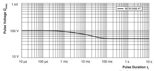
Maximum pulse voltage, single and continuous pulses; applicable if  $\hat{P} \leq \hat{P}_{max}$ ; for permissible resistance change equivalent to 8000 h operation in standard operation mode
