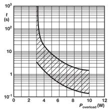
**NFR25** This graph is based on measured data which may deviate according to the application. Fusing Characteristics: 1  $\Omega \le R \le$  15  $\Omega$
