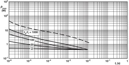
**NFR25** Pulse on a regular basis; maximum permissible peak pulse power ( $\hat{P}_{max}$ ) as a function of pulse duration ( $t_i$ ), 15  $\Omega \le R \le 15$  k $\Omega$
