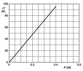
**NFR25** Hot-spot temperature rise ( $\Delta T$ ) as a function of dissipated power
