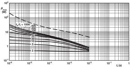
**NFR25** Pulse on a regular basis; maximum permissible peak pulse power ( $\hat{P}_{max}$ ) as a function of pulse duration ( $t_i$ ), 0.22  $\Omega \le R < 15 \Omega$
