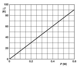
**NFR25H** Hot-spot temperature rise ( $\Delta T$ ) as a function of dissipated power
