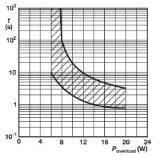
**NFR25H** This graph is based on measured data which may deviate according to the application. Fusing Characteristic: 1  $\Omega \le R \le 15 \text{ k}\Omega$
