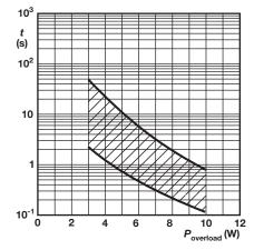
**NFR25** This graph is based on measured data which may deviate according to the application. Fusing Characteristics: 15  $\Omega \le R \le$  15 k $\Omega$
