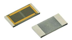
PCNM series chip resistors are designed on aluminum nitride ceramic substrates with enlarged backside terminations to reduce the thermal resistance between the topside resistor layer and the solder joint on the end users circuit assembly.
