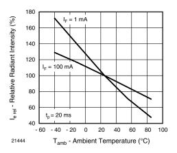
Fig. 6 - Relative Radiant Intensity vs. Ambient Temperature
