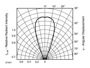
Fig. 8 - Relative Radiant Intensity vs. Angular Displacement
