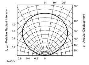
Fig. 6 - Relative Radiant Intensity vs. Angular Displacement
