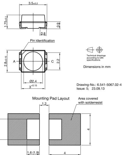
Dimensions: Reflow and vapor phase (wave soldering)
