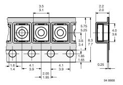
Fig. 9 - Tape Dimensions in mm for PLCC-2
