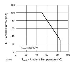
Fig. 2 - Forward Current Limit vs. Ambient Temperature
