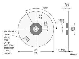
Fig. 11 - Dimensions of Reel-GS08
