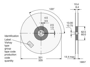
Fig. 12 - Dimensions of Reel-GS18
