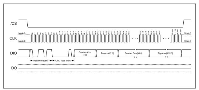
Figure 6. Increment Monotonic Counter Instruction
