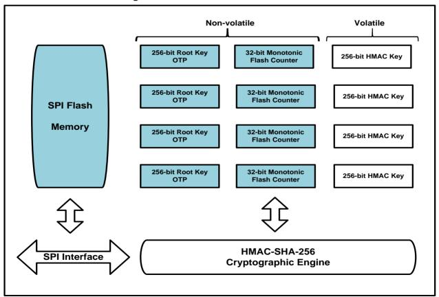
Figure 3. W74M12FV Functional Block Diagram
