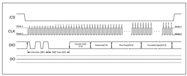
Figure 4. Write Root Key Register Instruction
