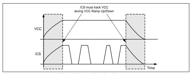
Figure 10b. Power-up, Power-Down Requirement
