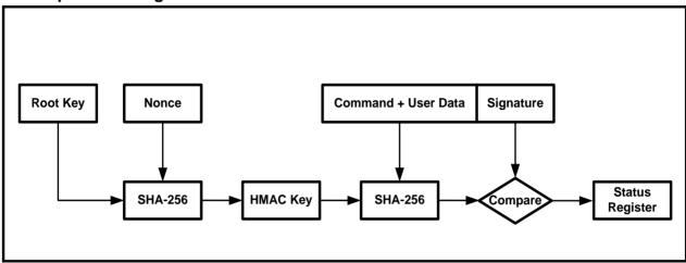
Figure 2. W74M12FV Operation Diagram
