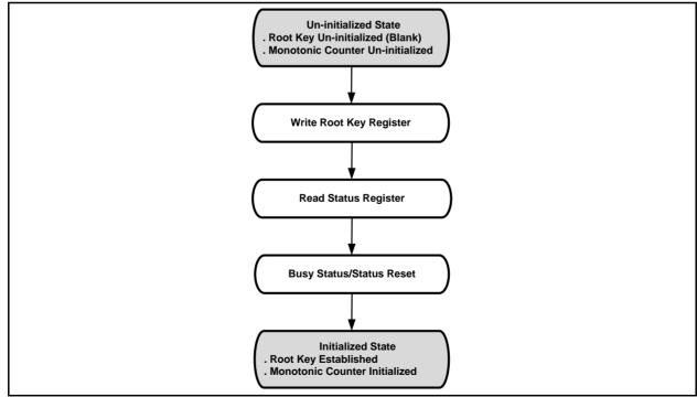
Figure 3a. W74M12FV Initialization Flow Diagram
