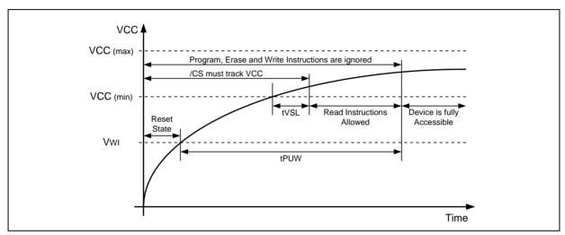
Figure 10a. Power-up Timing and Voltage Levels
