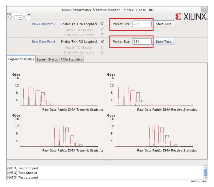
Figure 25: Effect of Varying Packet Sizes on Performance
