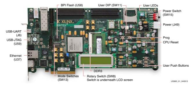
Figure 1: KC705 Board Features Used by the BIST
