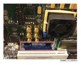
Figure 12: KC705 Board Plugged into a PCle x16 Slot
