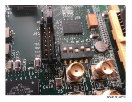
Figure 2: BIST Switch and Jumper Settings
