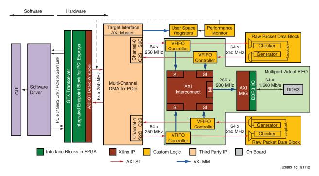
Figure 10: Kintex-7 FPGA Base TRD Block Diagram
