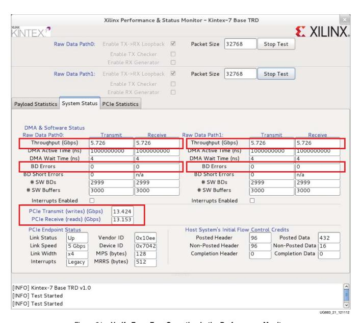
Figure 21: Verify Error-Free Operation in the Performance Monitor
